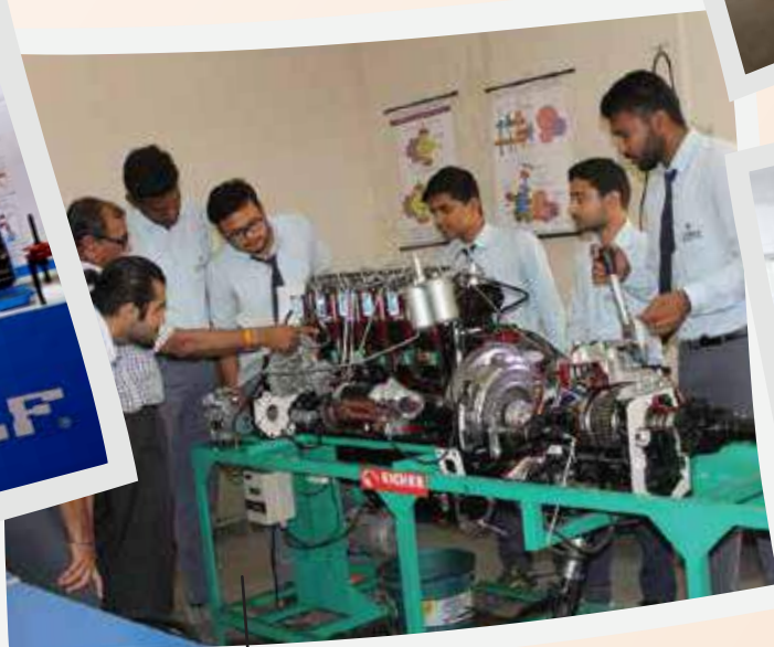
Eicher Cut Section Model Engine
